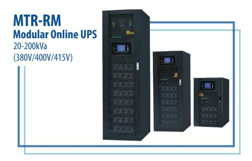
MTR-RM series is modular online UPS for sensitive equipments. The single cabinet power rating covers from 20KVA to 200KVA which delivers the best of combination of reliability, hot-swappable and flexibility. With the latest IGBT three-level technology and DSP control, MTR-RM achieves a high input power factor, low THD and high system efficiency, which make it a great choice for data centers, computer systems and critical equipments.
