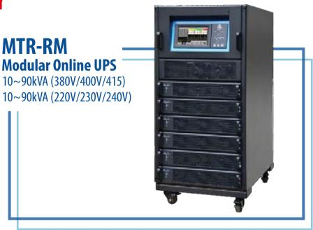
The rack modular, scalable, hot-swappable, online double conversion UPS ranging from 10 to 90kVA, with its flexible configuration of 3/3, 3/1 and 1/1, compact structure, is the ideal choice for small and medium data center.
